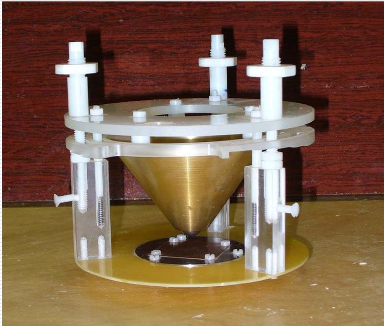
The cone with the angle  $70^\circ$  is made of brass and placed over the steel plate with the tungsten electrode.
