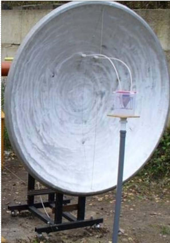
The antenna is placed at the focal point of the dish reflector 1.6 m in diameter. A convergent mirror is used for optimization of the antenna yield. The dish reflector and convergent mirror direct and amplify the signal from the antenna in the prescribed direction simultaneously keeping it off electromagnetic pulses from other sources (for example, discharge gaps of the Marx generator).
