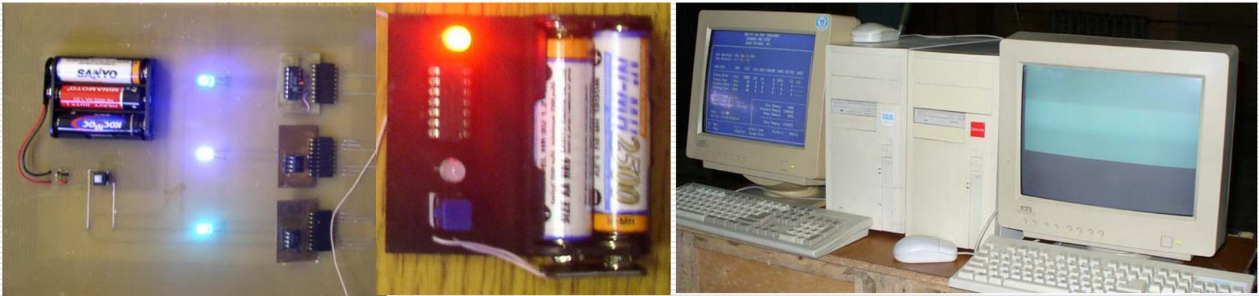
Test objects are the elements of analog and analog-digital dynamic circuits (for example, relaxation oscillator) specially developed for such experiments. LEDs in these circuits make circuit drop-in visible.
