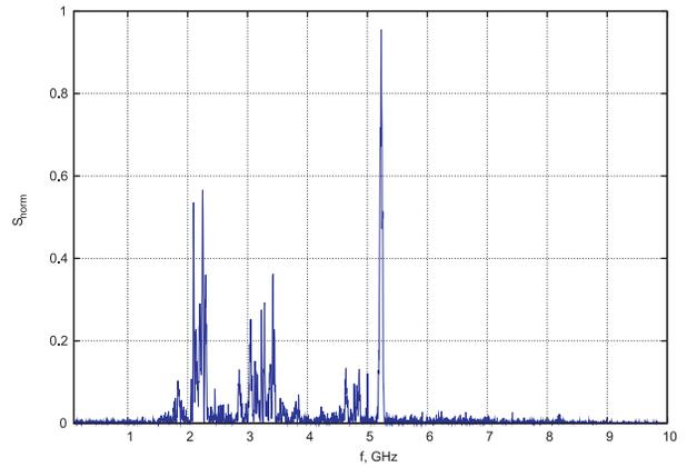
Figure 6: Radiation spectrum obtained by fast Fourier transform of the signal from the antenna for 0.8-18 GHz range.
