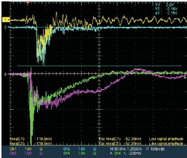
Figure 4: A typical signal from a TDS5 oscilloscope: diode voltage - green curve, diode current - magenta curve, blue and yellow - microwave signals.
