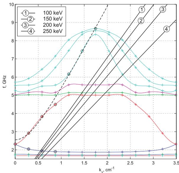
Figure 3: Dispersion properties of the foil photonic crystal.
