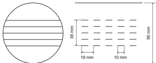
Figure 1: Foil photonic crystal design.
