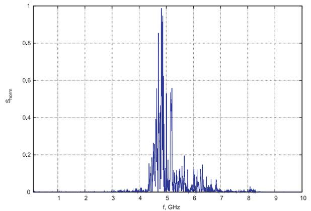
Figure 7: Radiation spectrum obtained by fast Fourier transform of the signal from the antenna for 4-8 GHz range.
