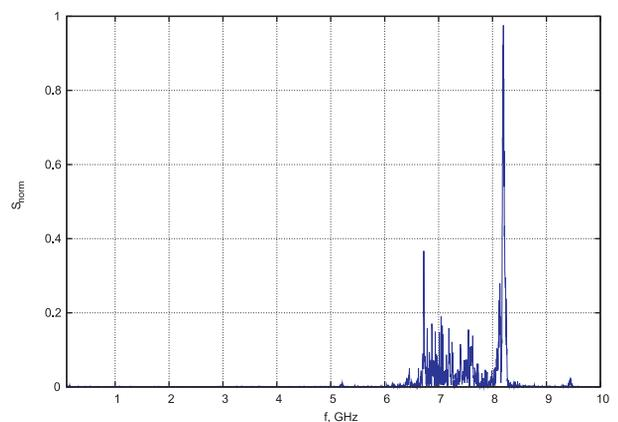
Figure 8: Radiation spectrum obtained by fast Fourier transform of the signal from the antenna for 8-12 GHz range.
