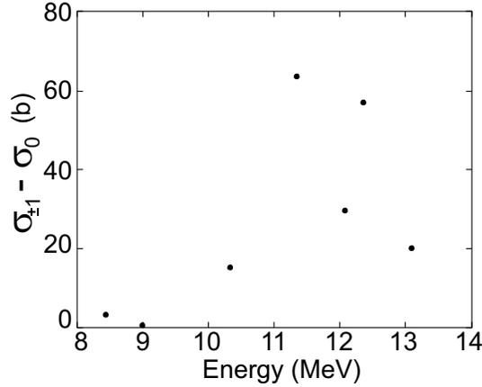
Fig. 2: Dependence of averaged effective difference of total cross-section  $\sigma_{\pm 1} - \sigma_0$  on averaged deuteron energy inside carbon targets obtained in experiments [3], [4].
