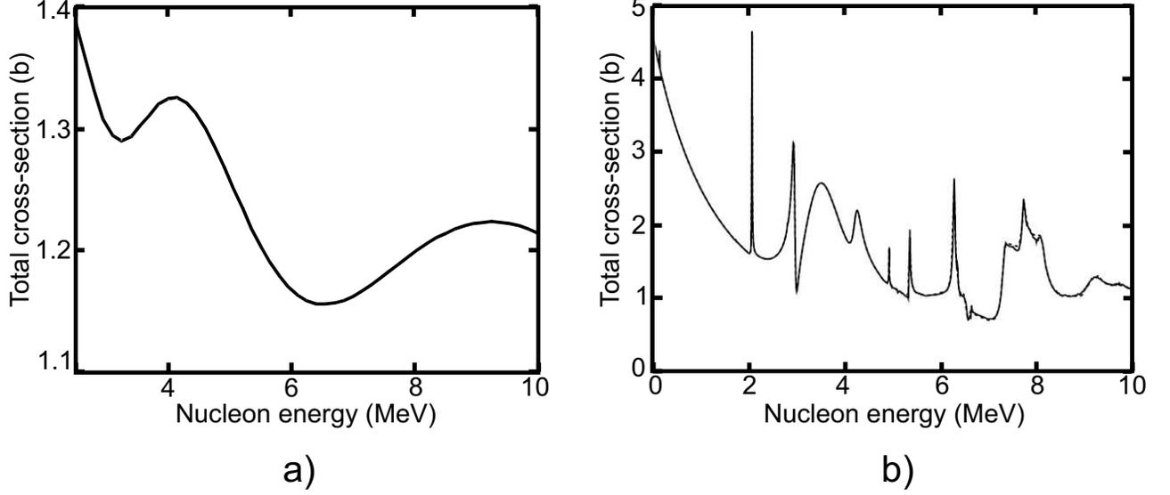
Fig. 3: Dependencies on nucleon energy of total nucleon-carbon cross-section calculated by a) eikonal approximation and b) from experimental data.
