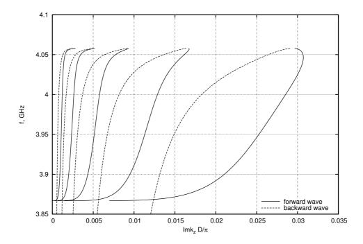
FIG. 2: The growth of the increment with beam current increase. On the graph are shown the increments for cases when the beam current is 0.1 A, 1 A, 10 A, 0.1 kA and 1 kA.
