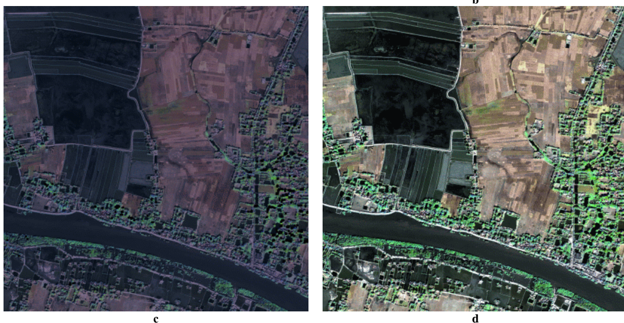
Fig. 6 – a – Original multispectral imagery in natural colors (Quickbird), b – four time pan-sharpening by our approach based on global regression (maximal original color preservation), c – Brovey pan-sharpening (big color distortion), d – pan-sharpening via HSV color space (small color distortion).
