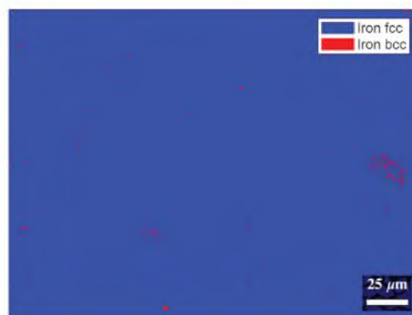
Fig. 2. EBSD phase map (austenite – Iron fcc and martensite – Iron bcc) of the implanted SS316L
