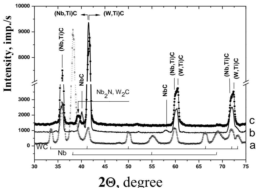
Fig. 1. Diffraction patterns of the Nb/hard alloy system after CPF treatment with 5 pulses at nitrogen pressure of 3 Torr with voltages of:
