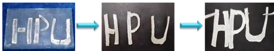
Figure 6. Digital photographs of the PG3 DN GPE excellent self-healing ability.
