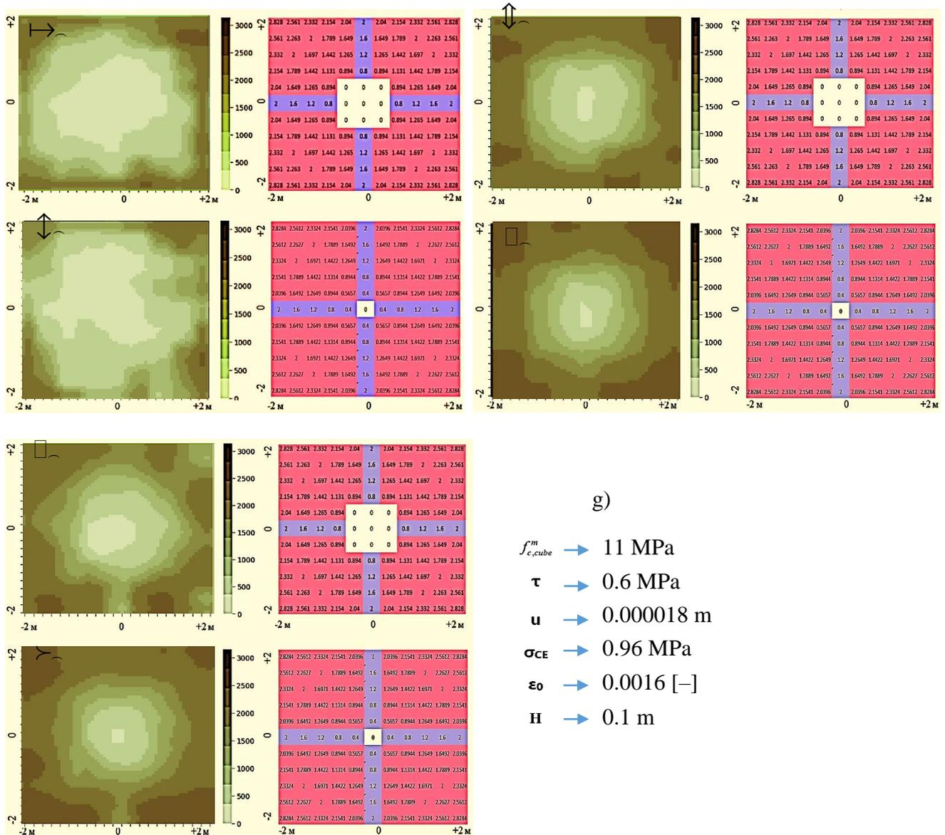
**Figure 6 – Displacements in slabs with central holes:**
