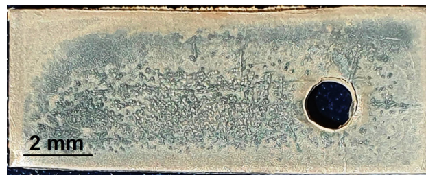
Fig. 4 A typical image of the oxidized samples (as-received, air, 180 secs)
