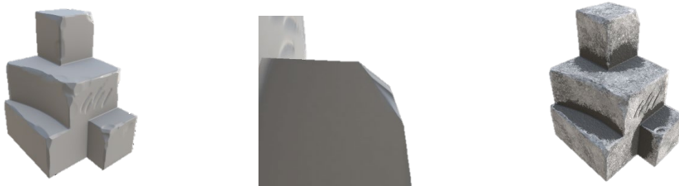
Fig. 6. 1 – the baked low-poly model; 2 – sharp ages on the baked low-poly model; 3 – the baked low-poly model with the textures assigned
