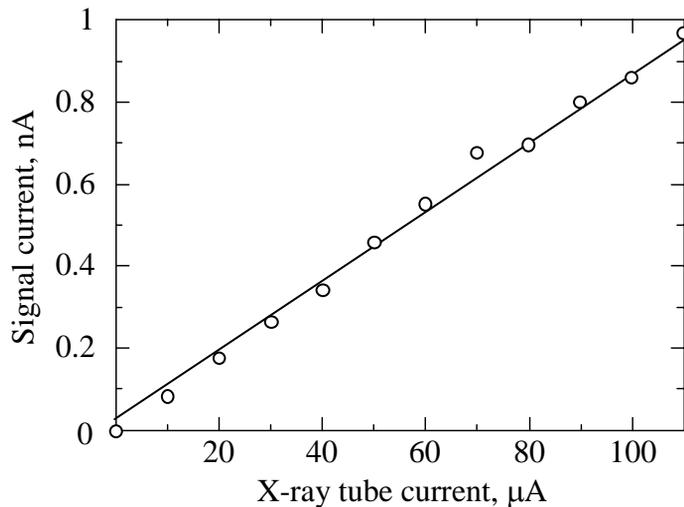
*Fig. 3.* The signal current as a function of the X-ray tube current
