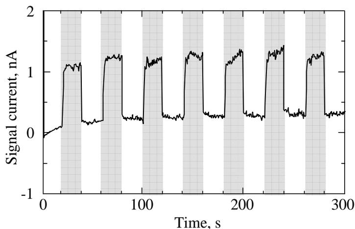
*Fig. 2.* The difference of the anode current in dark and X-ray irradiated conditions (experiment 1)
