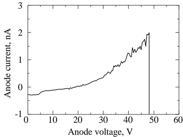
*Fig. 1.* The dark anode current as a function of applied anode voltage when field emission electrons irradiated CdTe
