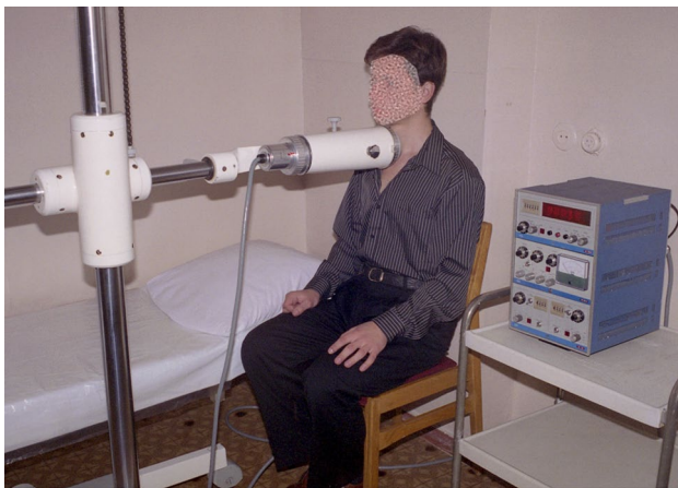
Fig. 5 Gamma-spectrometer NK and individual during ^{131}\text{I} thyroid activity measurement
