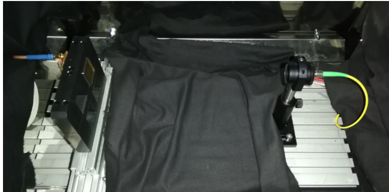
Figure 2. Calibration bench : PMT (left) and laser fiber on support (right).
