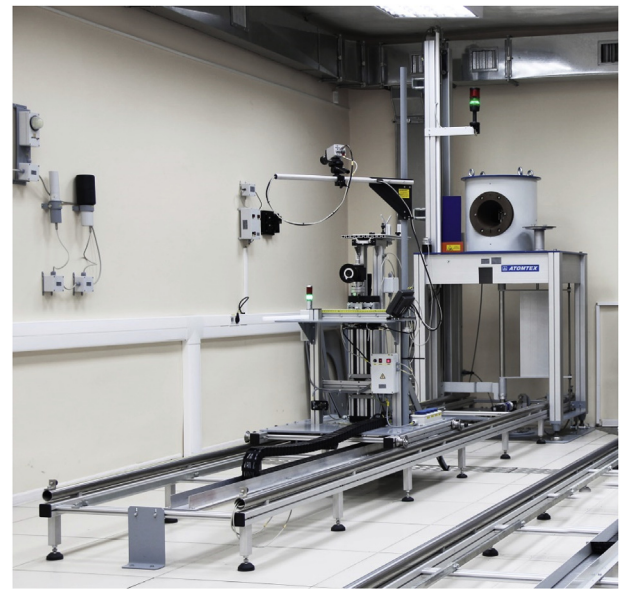
Fig. 7. Atomtex neutron irradiation facilities with reference neutron dosimetry bench AT140.
