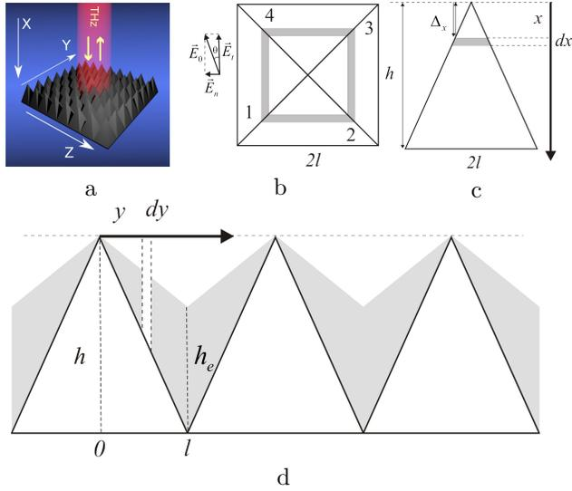
**Figure 2.** Backscattering of plane wave from pyramidal array. (a) Pyramidal array reflecting the terahertz radiation, (b) top view, (c) side view, (d) schematic image of pyramidal array covered with dielectric polymer.
