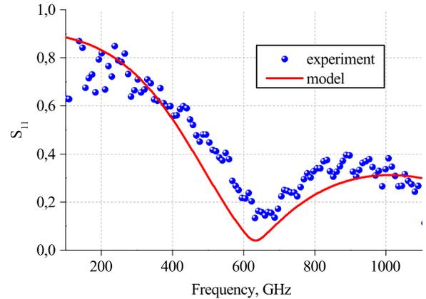
**Figure 5.** Amplitude of back-reflected signal  $S_{11}$  from periodic pyramidal CNT-array covered with epoxy resin layer (symbols correspond to the experimental data, line — to the modeling results).
