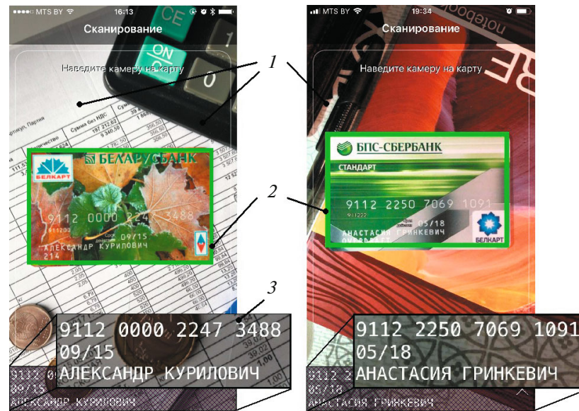
Fig. 2. Interface of the mobile application that implements the proposed algorithm: (1) viewing area, (2) mark of successful card detection, and (3) output area for recognized data.
