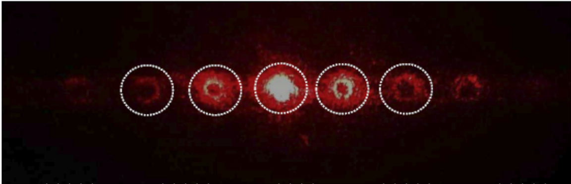
FIG. 3: (color online) Diffraction pattern of a Gaussian beam at the output of the one-dimensional fork-dislocation PLC grating.
