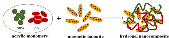
Fig. Schematic diagram for the synthesis of hydrogel nanocomposite based on magnetite-laponite
