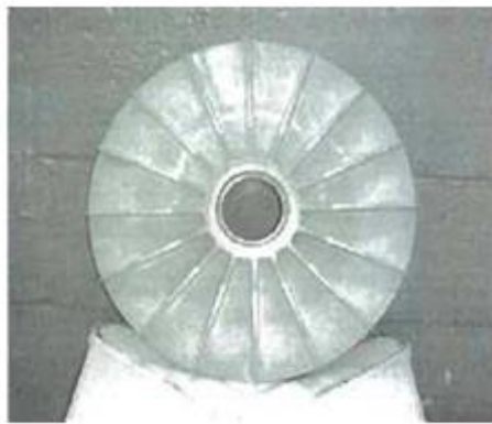
Fig 3.7.2. Turbine compressor, front view.
