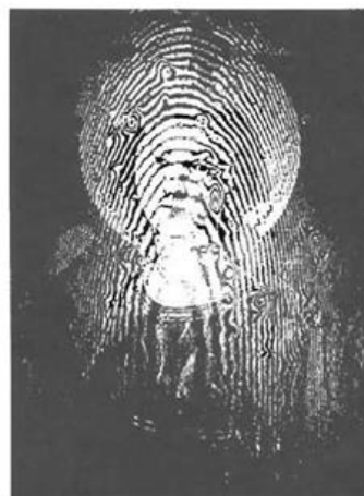
Fig 3.7.7. Holographic Interferogram made using thermal-drift method, revealing detachments.
