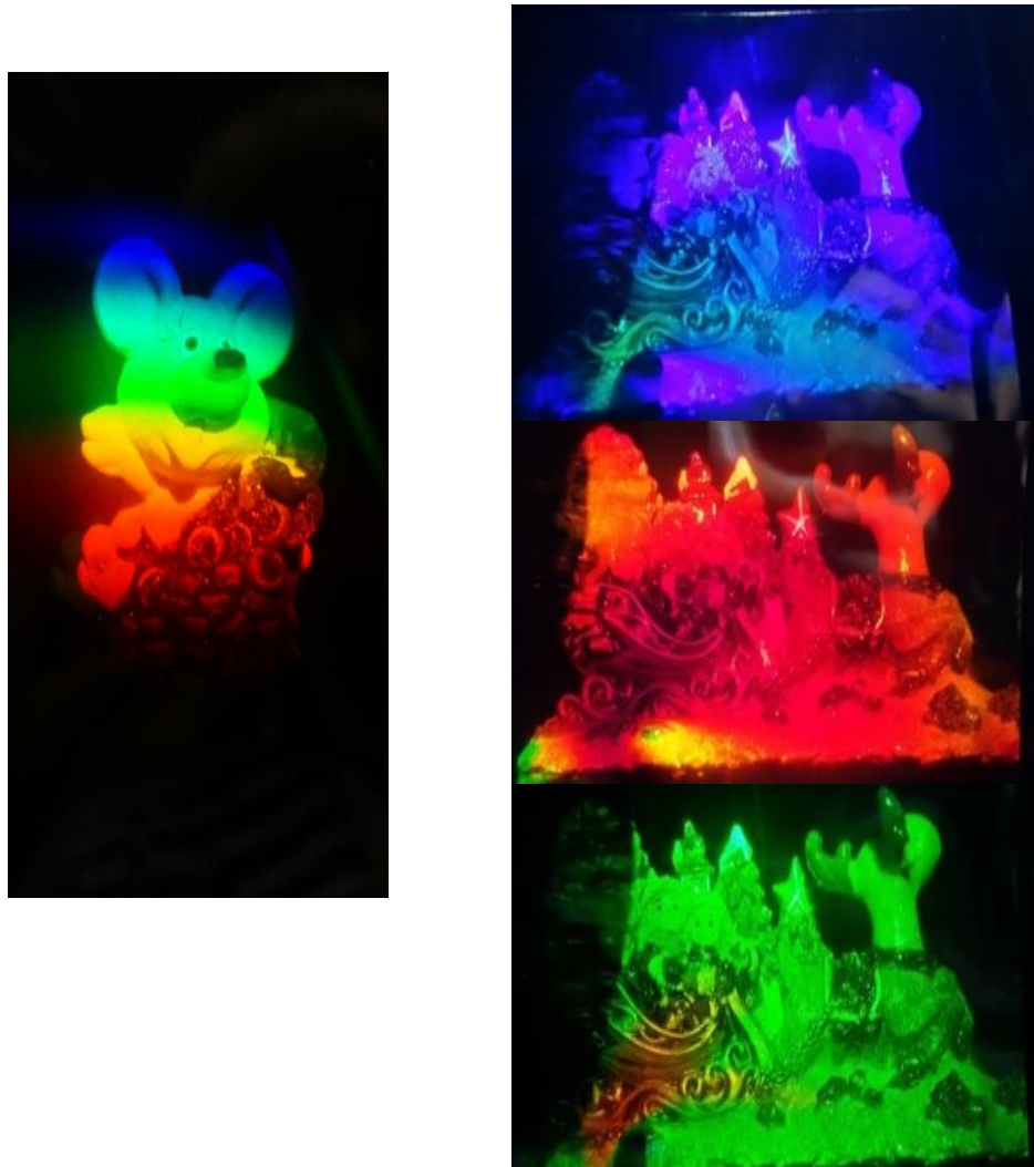
Figure 3.5.8- Images reconstructed from an iridescent hologram
