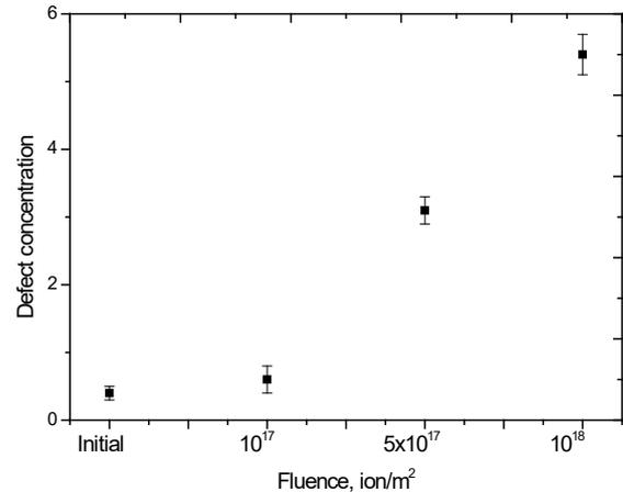
Fig. 2. Dependence graph of defect concentration in the structure on irradiation fluence
