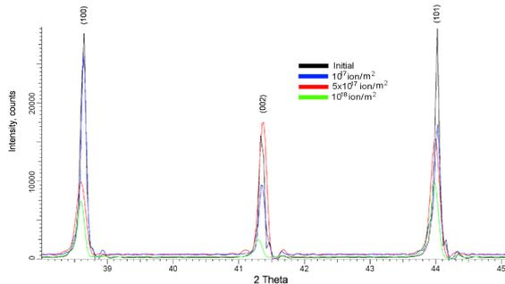
Fig. 1. Dynamics of changes in main diffraction maxima as a result of irradiation
