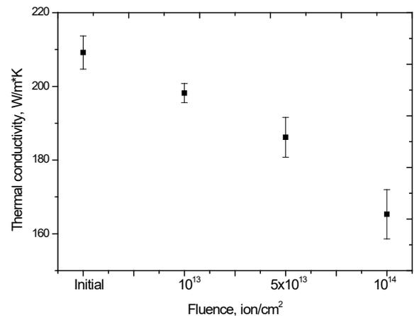
Fig. 3. Dependence graph of change in the thermal conductivity coefficient on irradiation fluence
