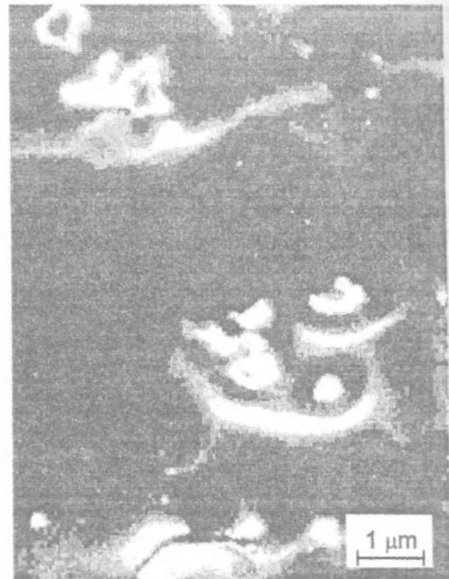
Fig. 3. Scanning electron microscope image of glass microparticles sputtered with sample rotation technique. Hollow surfaces in indium carrier surround the particles.
