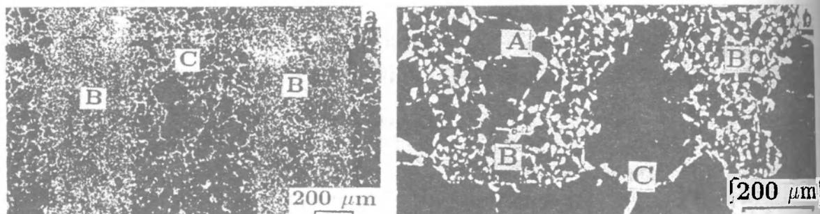
Fig.2. Structural changes in the regions of the U7 steel sample irradiated with alpha-particles by the method 2 and annealed at 900°C. a - structure of bombarded surface, b - structure along the direction of alpha-particle motion., A - region of irradiation-for "shooting through", B - helium doped region, C unirradiated region.
