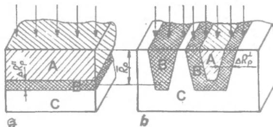
Fig.1. The scheme zones production in samples of the U7 steel irradiated with high-energy particles by the method 1 (a) and method 2 (b): A - the region of alpha-particles (proton) "shooting through", B - the helium (hydrogen) doped region, C - unirradiated region,  $R_p$  - projective range of charged particles,  $\Delta R^{\parallel}$  - longitudinal straggling,  $\Delta R^{\perp}$  - lateral straggling.
