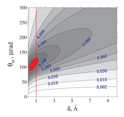
FIG. 8: Measure in centimeters average length  $\langle \Delta z \rangle$  of scattering of particles entering the crystal through the lateral crystal surface vs both miscut angle and diffusion step at perfect crystal plane alignment.
