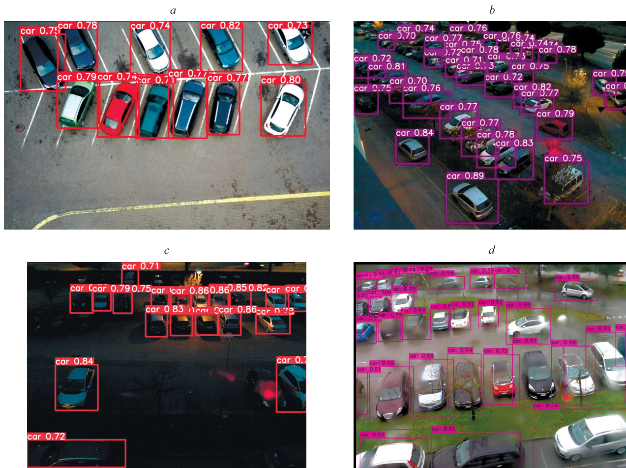
Fig. 5. Car detection results on a sunny day (a), in the evening (b), at night (c), on a rainy day (d)
