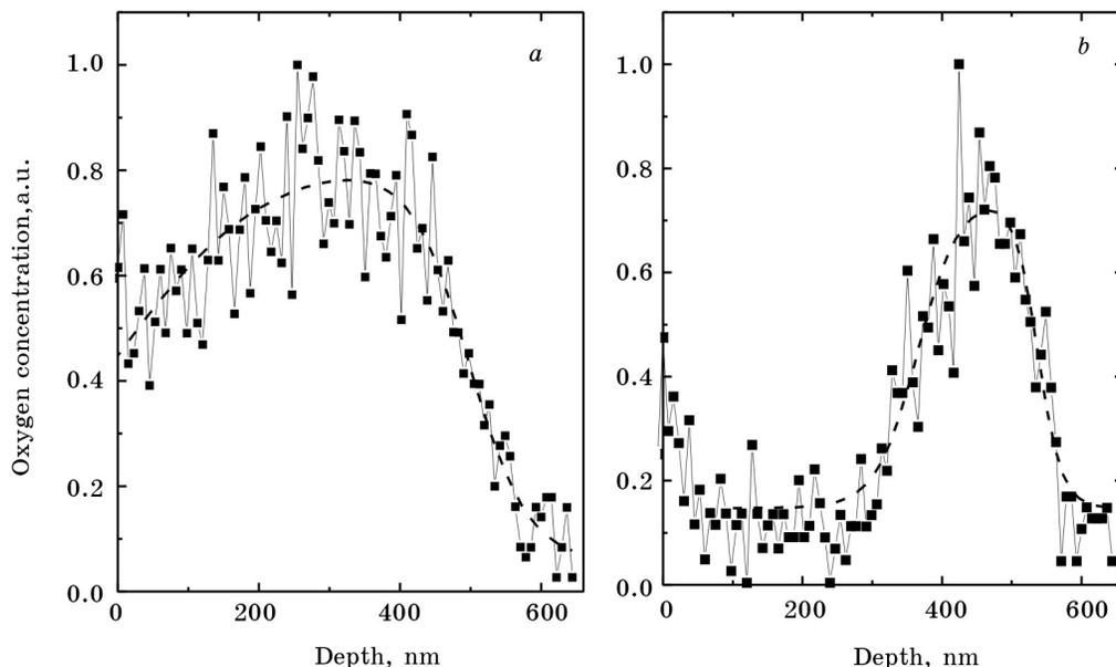
Fig. 2. Oxygen depth profiles for polyethylene implanted with (a)  $10^{16}$  B<sup>+</sup>/cm<sup>2</sup>, (b)  $5 \times 10^{16}$  B<sup>+</sup>/cm<sup>2</sup> at 100 keV. The depth profiles are reconstructed from the RBS spectra
