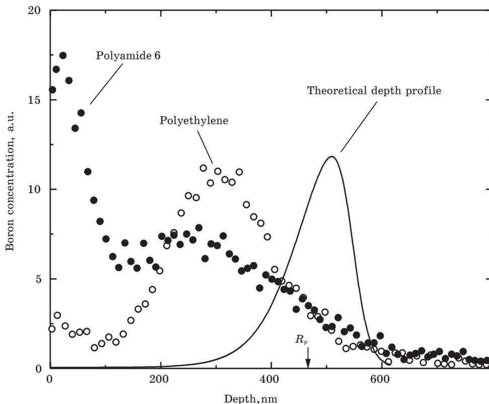
Fig. 3. Boron depth profiles for polyethylene and polyamide 6 implanted with  $5 \times 10^{16} \text{ B}^+/\text{cm}^2$  at 100 keV. Theoretical depth profile for boron implanted into polyethylene was calculated by TRIM code,  $R_p$  is the theoretical projected range
