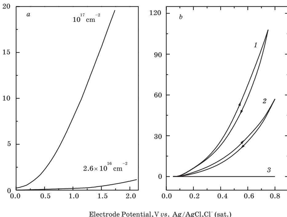
Fig. 7. Polarization curves for oxidation of (a)  $10^{-1}$  M hydroquinone at polyamide 6 implanted with 100-keV  $B^+$  to different doses; (b)  $2 \times 10^{-2}$  M ortho-phenylenediamine at polyethylene implanted with 100-keV  $B^+$  to a dose  $10^{17} \text{ cm}^{-2}$ : the first cycle (curve 1), the second cycle (curve 2), the tenth cycle (curve 3). Supporting electrolyte is 0.25 M  $\text{Na}_2\text{SO}_4$ .
