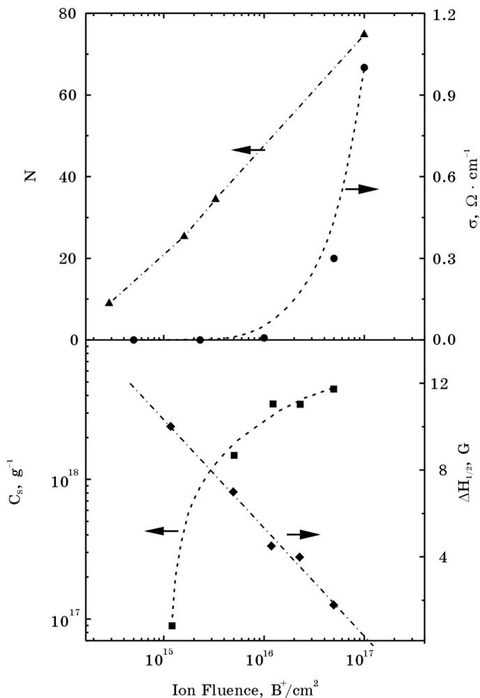
*Fig. 5.* The fluence dependence of the number of benzoid rings forming carbon cluster ( $N$ ), d.c. conductivity ( $\sigma$ ), spin concentration ( $C_s$ ) and the linewidth ( $\Delta H_{1/2}$ ) for polyethylene implanted with 100 keV  $B^+$ .
