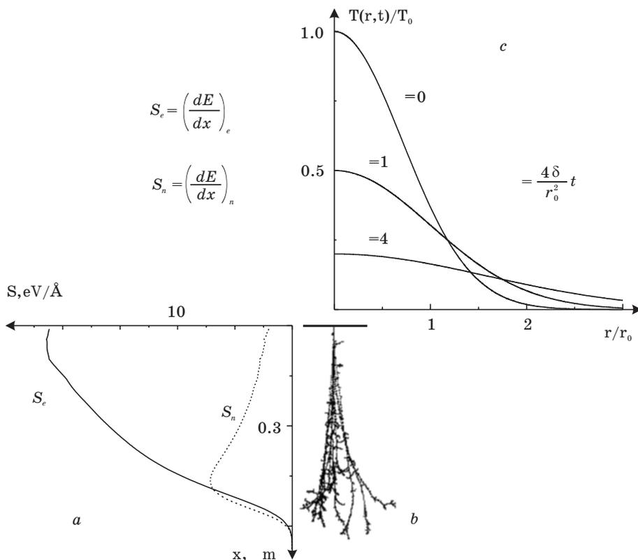
Fig. 1. (a) Energy loss parameters versus penetration depth and (b) trajectories of 100-keV  $B^+$  implanted into polyethylene (the Monte-Carlo simulations with the use of TRIM code); (c) temperature distribution in the ion track region and its evolution with time (in the dimensionless variables)
