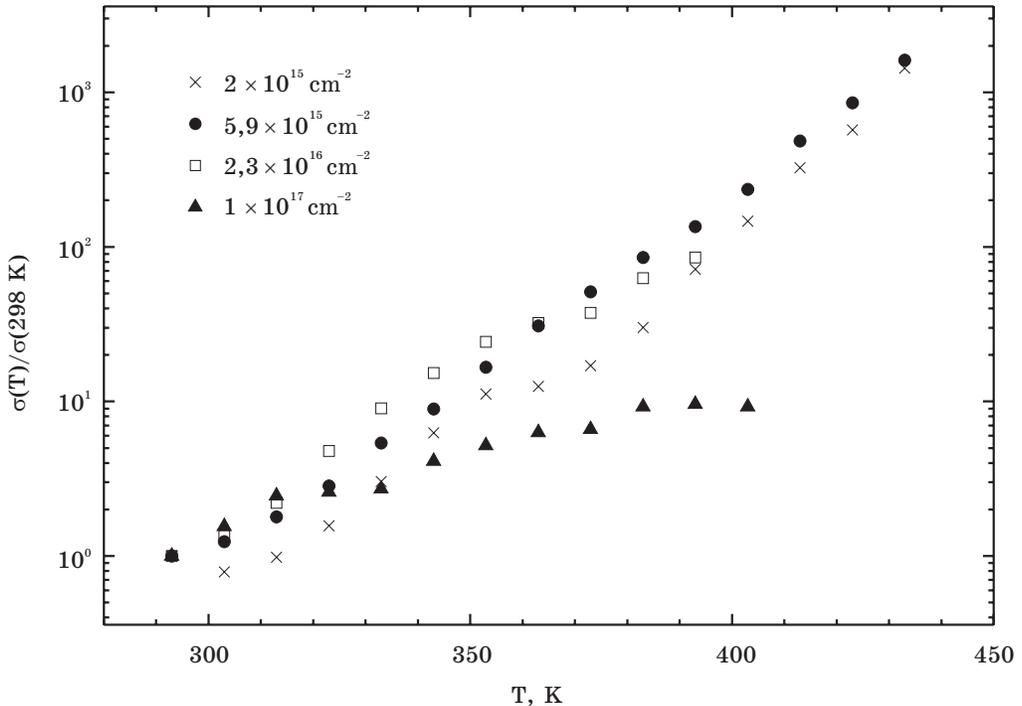
Fig. 6. Temperature dependence of d.c. conductivity for polyethylene implanted with 100 keV B<sup>+</sup> to different doses
