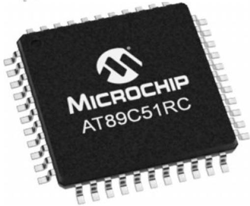
44 44A – TQFP (Thin Plastic Gull Wing Quad Flatpack)
