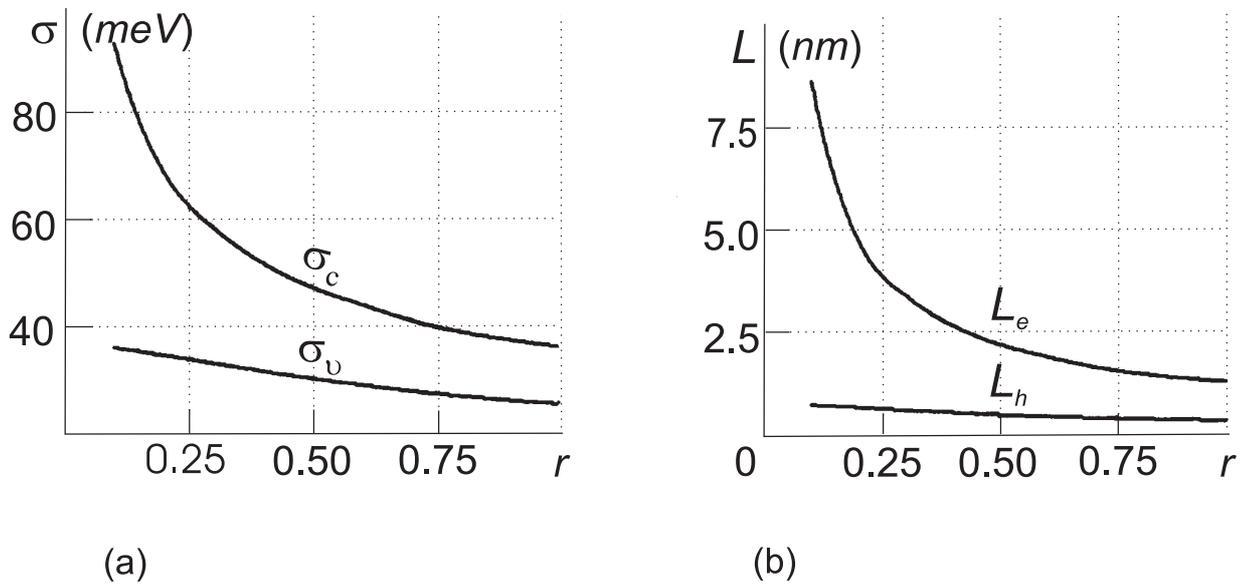
FIG.2. (a) Parameters of density state tails  $\sigma = \sigma_c$  or  $\sigma_v$  and (b) screening lengths  $L = L_e$  or  $L_h$ , in  $n$ - or  $p$ -regions, respectively, versus the pump factor  $r$ .  $N_a = 10^{19} \text{cm}^{-3}$ ,  $N_d = 6 \times 10^{-18} \text{cm}^{-3}$ ,  $d_n = d_p = 15 \text{nm}$ ,  $d_i = 0$ ,  $T = 300 \text{K}$ .
