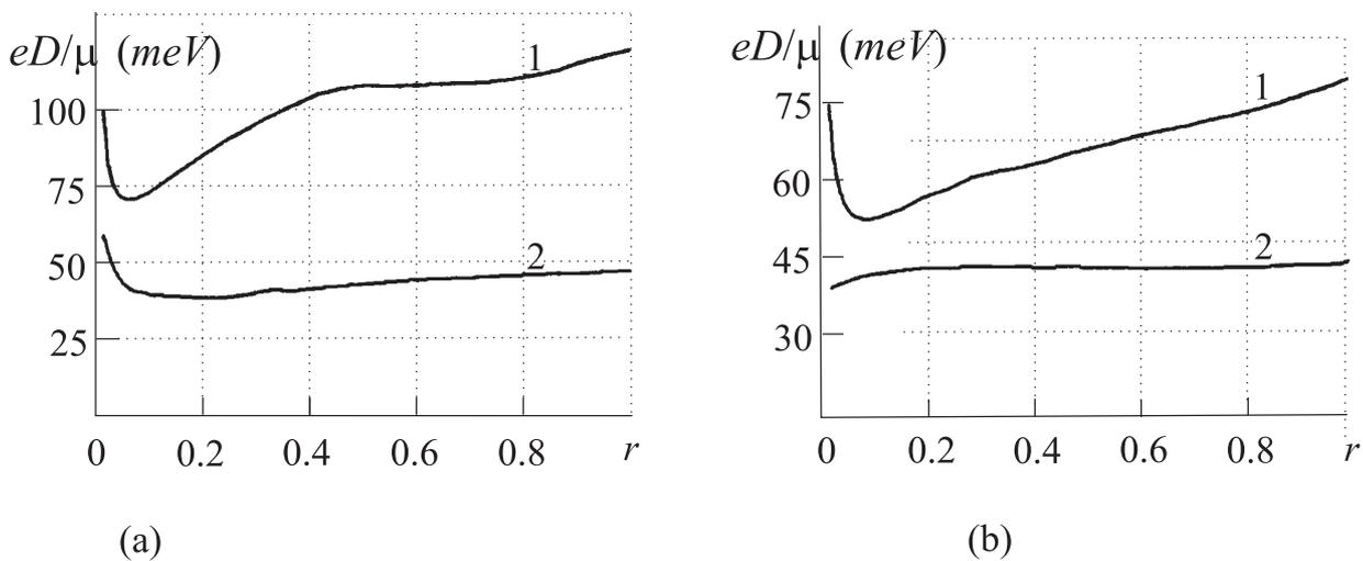
FIG.3. Diffusivity-mobility ratio for (1) electrons and (2) holes versus the pump factor  $r$ . (a)  $N_a = N_d = 10^{19} \text{cm}^{-3}$  (b)  $N_a = 10^{19} \text{cm}^{-3}$ ,  $N_d = 5 \times 10^{18} \text{cm}^{-3}$ ,  $d_p = d_n = 15 \text{nm}$ ,  $d_i = 0$ ,  $T = 300 \text{K}$ .
